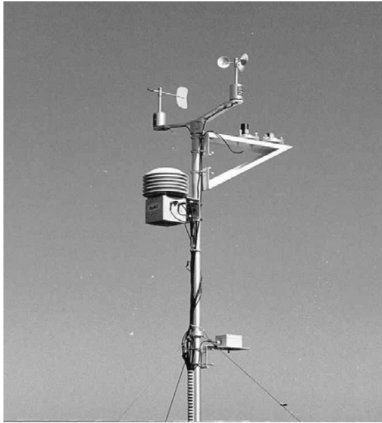
Figure 10. Automatic meteorological station MiniMet in operation at the Kishinev site
