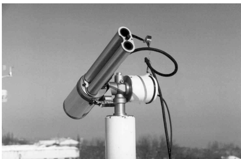
Figure 1. Sunphotometer CIMEL CE-318 in operation at the Kishinev site (47.00°N, 28.82°E; 205 m a.s.l.).
